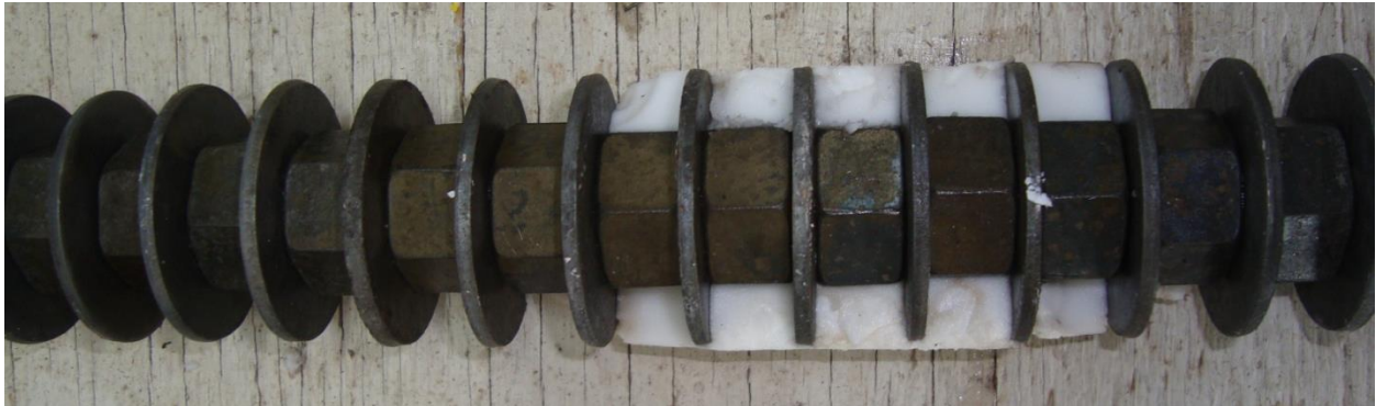
Figure 4 - Labyrinth mandrel produced a 400 psi medium pressure seal
