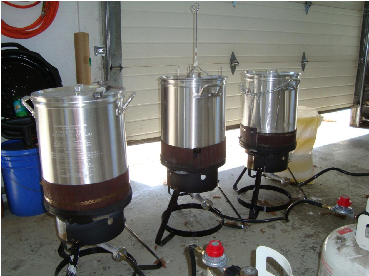
Figure 2 Heating vessels insulated to minimize heat loss
