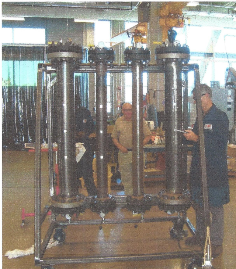
SAIT ARIS technician measuring 7" test spool diameter
