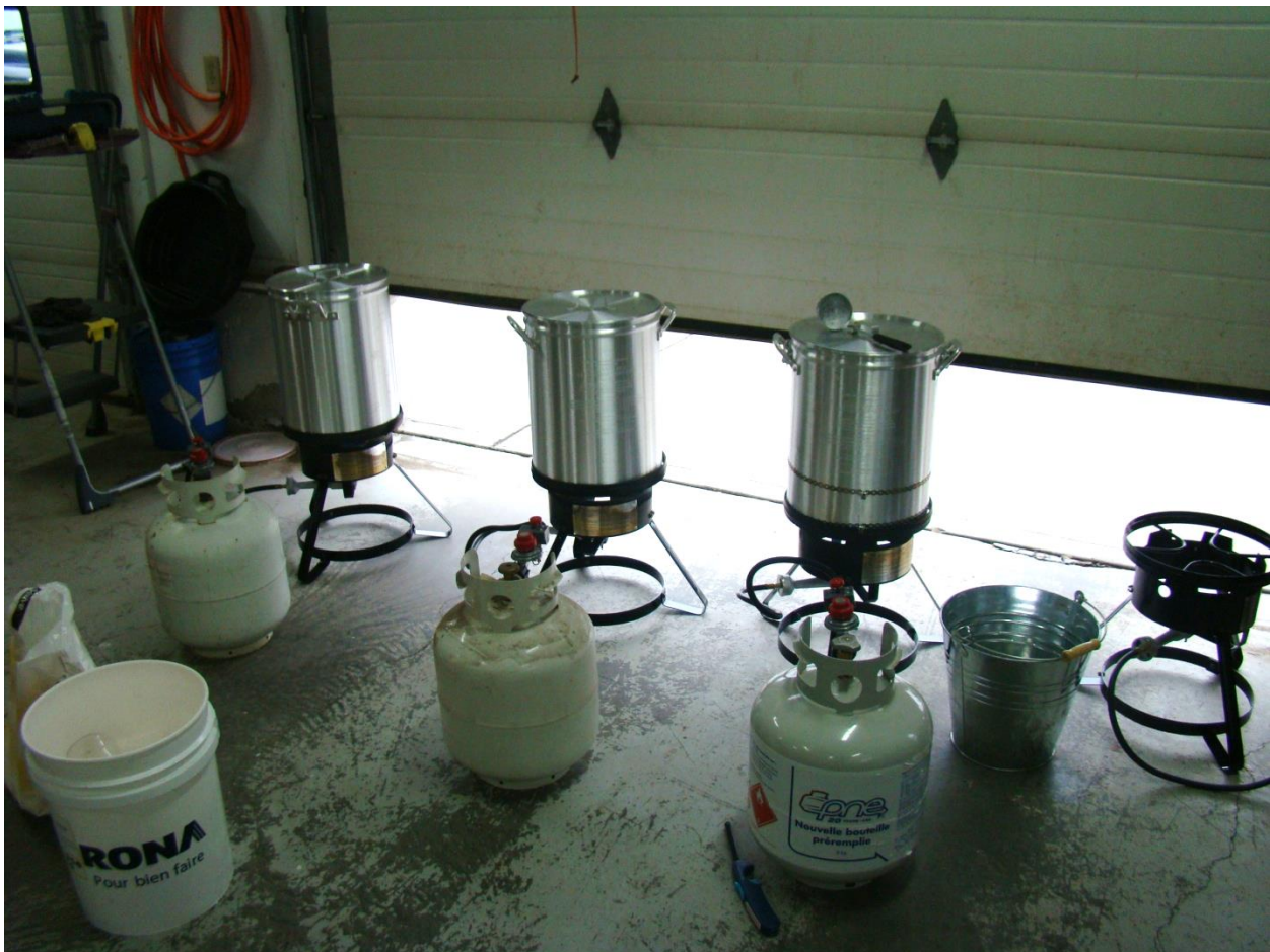
Figure 1- Propane fired heaters melting salt
