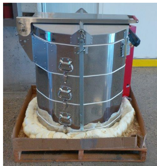
Electric kiln used to melt eutectic salt
