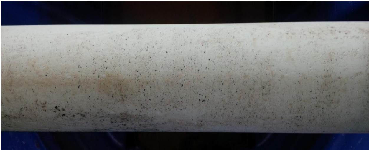
Figure 1 - Porous surface on salt column caused by entrained vapour "bubbles"
