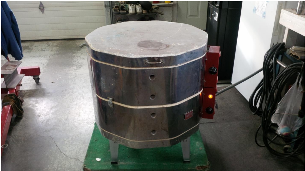
Figure 3 - Electric kiln provides better control of salt melting
