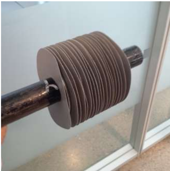
Dry assembly of 4.5" seal elements
